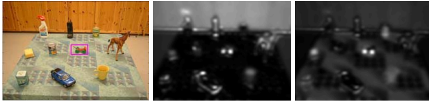
Fig. 14: An example of successful optimization; the ROI is marked in the left image. Without optimization (unitary weights) the saliency map is purely Bottom-up (middle). However, an optimization that minimizes e_{ROI}(\bar{\omega}) (in this case to 0) the optimal weight vector \bar{\omega}_{opt} clearly ranks the ROI as the best hypothesis of the Top-down map (right).
