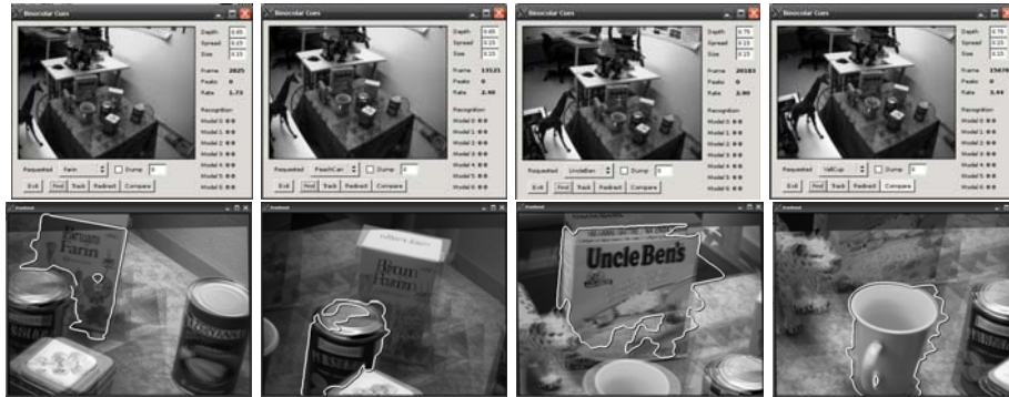
Fig. 19: The visual frontend. The top row shows the widefield view where the visual search selection is made. The bottom row shows the foveal view in which the binocular segmentation and recognition as well as validation is done.
