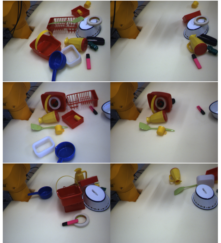
Fig. 15. Complex scenes 1, 2 and 3. Images on the left show initial scenes. Images on the right show the corresponding scenes after 30 grasping attempts with our grasping behaviour.
