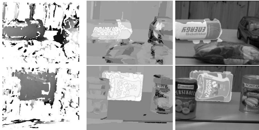
Fig. 8: Disparity maps (right), prior foreground probabilities (center) and posteriori figure-ground segmentation (left).
