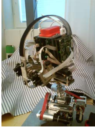
Fig. 3: The Armar-III stereo head.
