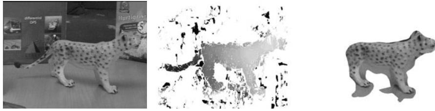
Fig. 12: Left) A left manipulation camera image, Middle) The corresponding disparity map, Right) Segmentation from mean shift in 3D space.
