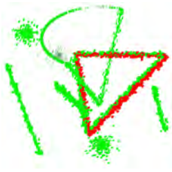
Fig. 7. Accuracy of pose estimation. The noisy triangle scene is green, and the red triangle indicates where the system estimates its position.
