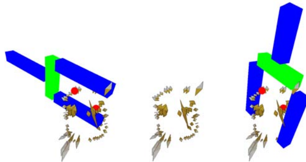
Figure 7.27: The wrong EGA 4 hypotheses (left) was performed, whereas the correct grasping hypotheses of type EGA 1 (right) was not because the approach configuration was unreachable by the robot.
