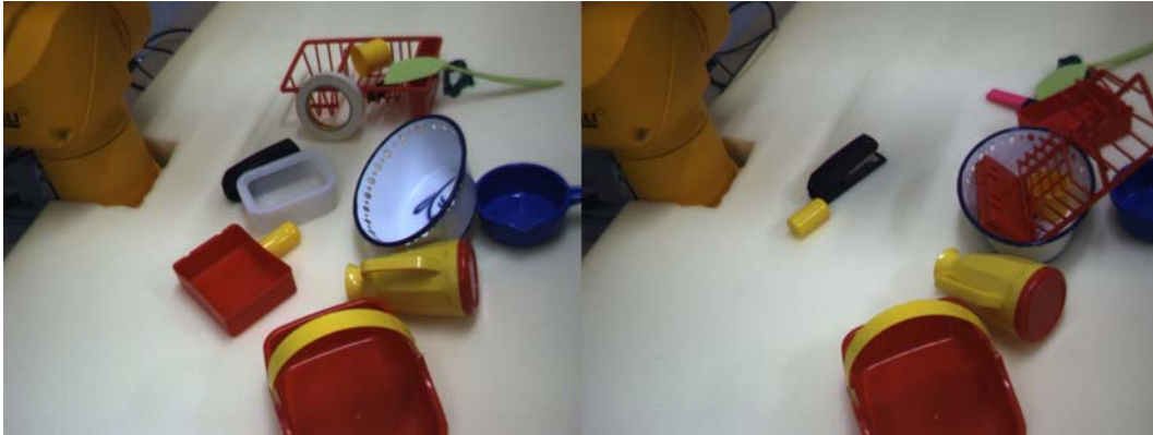
Figure 7.34: Complex scene 5. Left image shows the initial scene for both random grasping and grasping reflex experiments. The image on the right shows the scene after 30 grasping attempts with grasping reflex.
