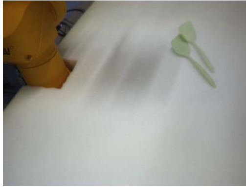
Figure 7.11: The Figure shows how an object is moved after unsuccessful grasping attempt. Following grasping attempts that are scheduled for execution before next exploration cycle are not any more valid.
