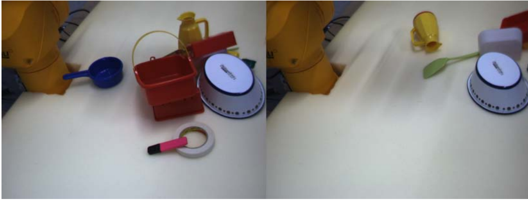
Figure 7.33: Complex scene 4. Left image shows the initial scene for both random grasping and grasping reflex experiments. The image on the right shows the scene after 30 grasping attempts with grasping reflex.
