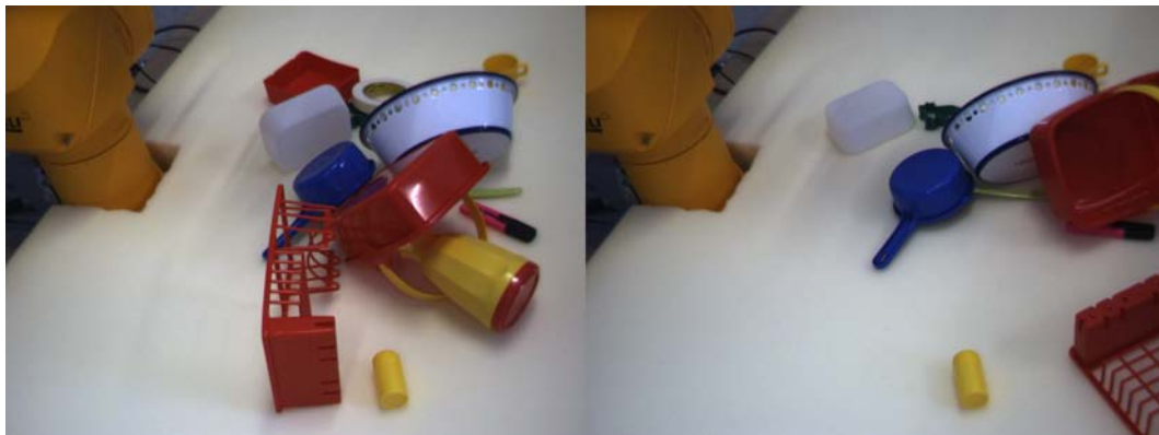
Figure 7.31: Complex scene 2. Left image shows the initial scene for both random grasping and grasping reflex experiments. The image on the right shows the scene after 30 grasping attempts with grasping reflex.
