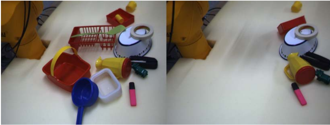
Figure 7.30: Complex scene 1. Left image shows the initial scene for both random grasping and grasping reflex experiments. The image on the right shows the scene after 30 grasping attempts with grasping reflex.
