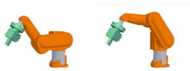
Figure 5.9: Two different robot configurations lead to the same tool position. The left image shows “elbow down” and the right image “elbow up” configuration.
