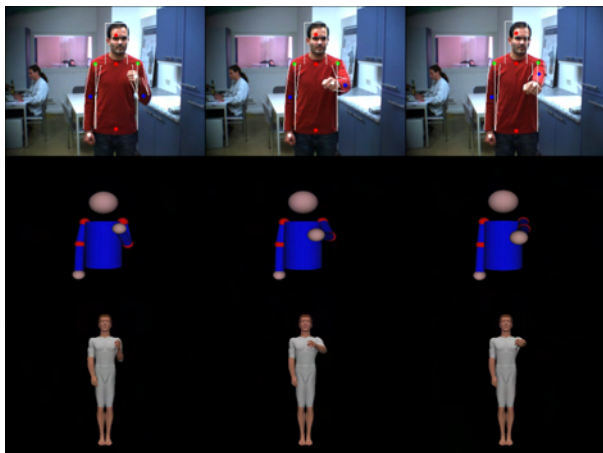
Fig. 5. Screenshots showing tracking performance. Top: input images of the left camera with projected estimation. Middle: Visualization with a simple 3D model. Bottom: Visualization by mapping to a realistic human model
