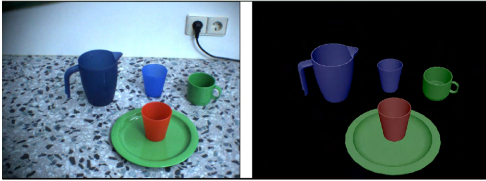
Fig. 6. Typical result of a scene analysis. Input image of the left camera (left) and 3D visualization of the recognition and localization result (right).
