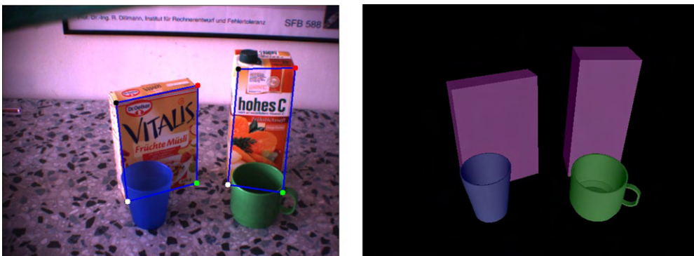
Fig. 8. Recognition and localization result for an exemplary scene. Input image (left) and 3D visualization of the result (right).
