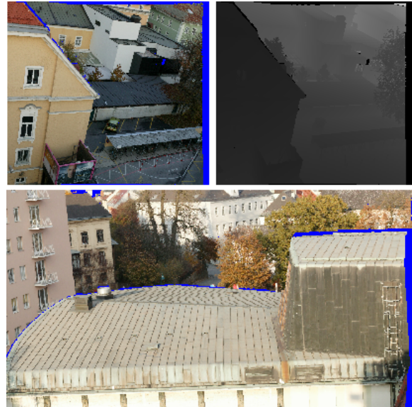
Figure 3: A subset of the 20 3D data sets used in the analysis. The points without corresponding range data are marked in blue. The gray image shows the range data of the top-left scene. The resolution range of the whole data set is [512-2048] \times [390-2290] with an average resolution of 1140 \times 1001 .
