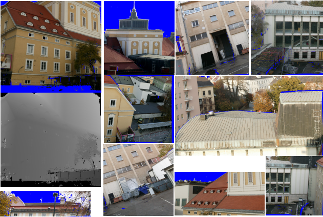
Figure 3. 10 of the 20 3D data sets used in the analysis. The points that don't have range data are marked in blue. The gray image shows the range data of the top-left scene. The resolution range is [512-2048]x[390-2290] with an average resolution of 1140x1001.
