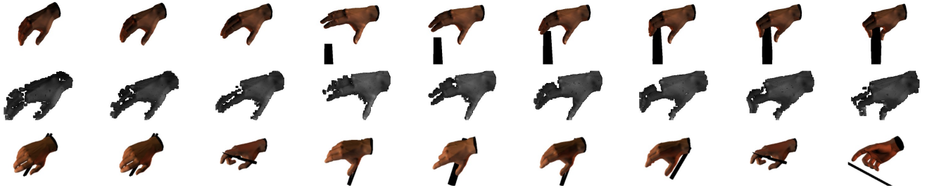
Fig. 6. Synthetic sequence 1. Top: original synthetic image. Middle: segmentation image with \alpha = 0.5\% . Bottom: estimated pose. (The objects in the database are colored black for visibility here, but do not contribute to the HOGs.) Video at www.csc.kth.se/~jrjn/VideosICRA2010/synthetic1.mp4
