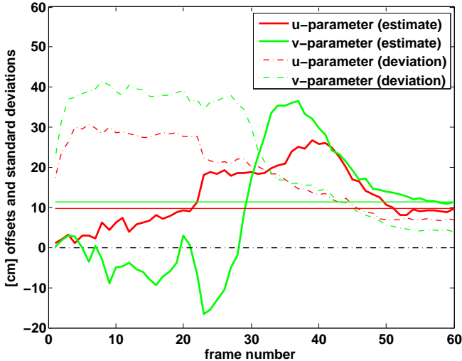
Fig. 12: Progression of Action Parameters. The figure shows the progression of the current estimate of the action parameters u, v over time, where (u, v) defines the pointed at position on table-top, and is measured as offset in cm to center of the active table-top region, in the images of Fig. 10 the variables correspond to the “horizontal” ( u ) and “vertical” direction ( v ). The dotted lines show the standard deviation for u and v .
