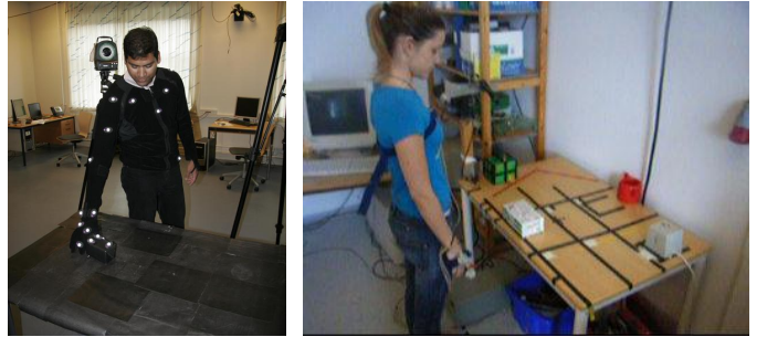
Fig. 5: Left: Our Experimental Setup . The markers are attached to both, person and object. The object can be moved from any position to any other position on the table. Right: Experimental Setup in [9] . The table is marked with locations where the object can be moved around. Object positions are not recorded.
