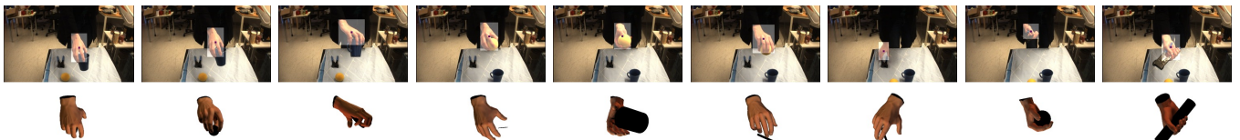
Fig. 12. Real sequence 3 (female subject 3). Top: image with skin segmentation window highlighted. Bottom: estimated pose. (The objects in the database are colored black for visibility here, but do not contribute to the HOGs.) Video at www.csc.kth.se/~jrgn/VideosICRA2010/real3.mp4
