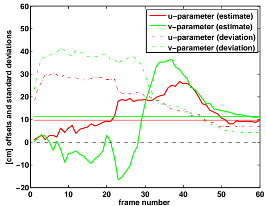
Figure 1. The figure shows the progression of the current estimate of the action parameters over time. The estimate parameters u, v are computed as mean of all particles \omega = (u, v, k) . The action parameters u, v correspond to the x-, and y-offsets to the center of the active table-top region (x corresponds to the horizontal, y to the deeps direction in Fig. 4). The dotted lines show the standard deviation of the particles.
