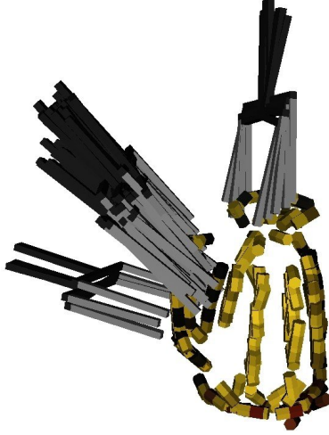
Figure 2: Grasp density. Each gripper represents a particle of its nonparametric representation; their density reflects the local grasp success likelihood.
