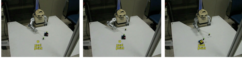
Figure 4: Pushing behavior realized by \text{oac}^{push} after learning transformation function \text{oac}^{push}.T^B
