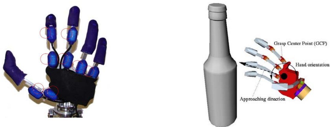
Figure 5: The used five-fingered anthropomorphic hand with eight independent joints (left) and a schematics with the grasp descriptors.
