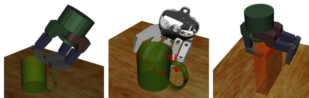
(g) Barrett 2-finger Thumb (h) Robonaut 4-finger Thumb (i) Failed Barrett Wrap
