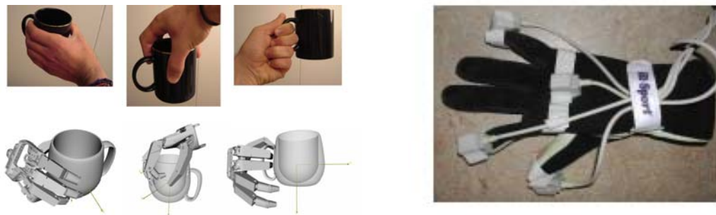
Figure 4: Different grasps are possible for picking up a cup (left) and the glove used for measuring human grasps.
