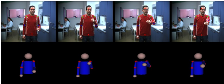
Figure 1: Example snapshots of a tracked image sequence. Top: Left input image with projection of the calculated configuration of the human model. Bottom: 3D visualization of the calculated configuration.
