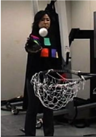
Fig. 2. The initial throwing behavior was captured and processed in real time using color markers attached to the body and computer vision techniques.
