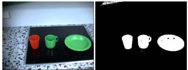
Fig. 8. Illustration of the color segmentation result for the colors red and green
