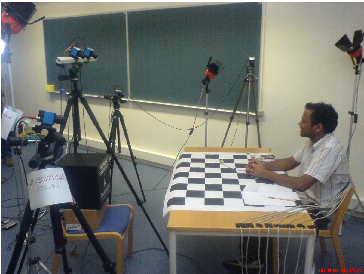
Figure 3: The image shows the setup of the recording session of the AAU dataset. One can see the four blue video cameras and the cables for the motion star system (bottom right). At the bottom left, the transmitter of the motion star system is visible.
