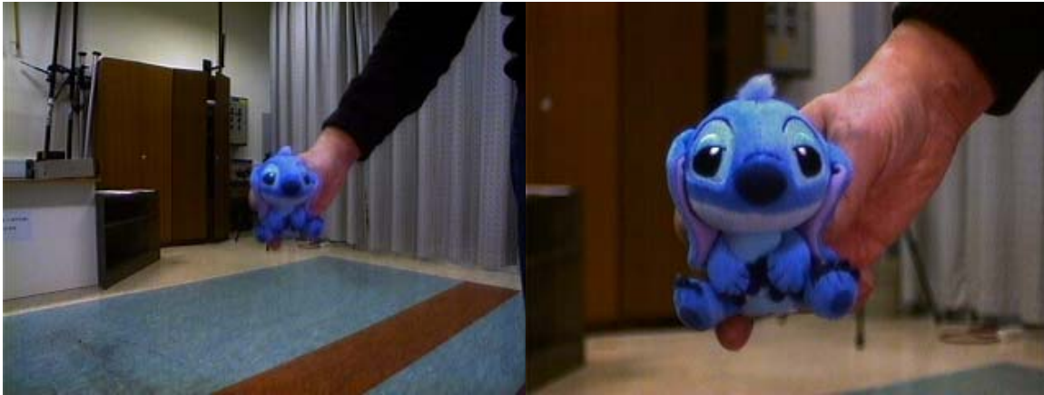
Figure 2. Simultaneous views from the peripheral and foveal cameras. The high resolution of object image and better localization makes foveal images suitable for image analysis task such as object recognition (right), while the wide field of view from the peripheral camera is suitable for visual search and smooth pursuit (left).
