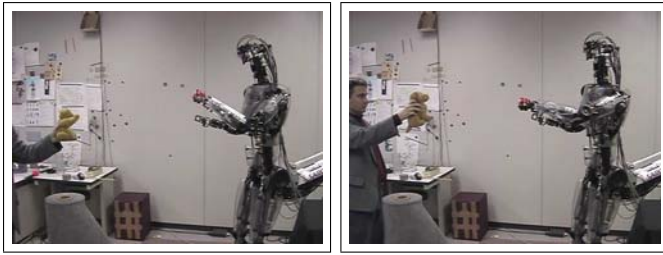
Fig. 10. DB in behavioral experiment. The task of the robot is to point towards the desired object (toy dog in the right image) and to ignore the rest of the objects.
