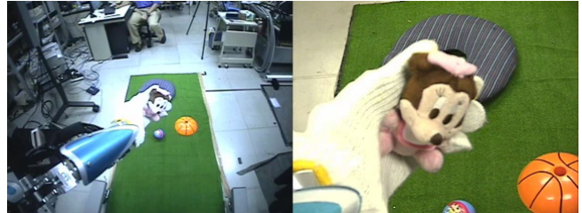
Fig. 1. Simultaneous view of the object from the peripheral and foveal camera of a humanoid robot. The images from foveal camera are used for learning object representations.
