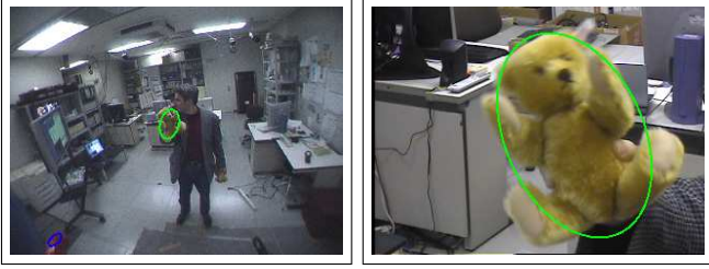
Fig. 2. Simultaneous views from the peripheral and foveal cameras. The high resolution of object image and better localization makes foveal images suitable for recognition (right), while the wide field of view from the peripheral camera is suitable for smooth pursuit (left).
