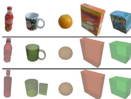
Figure 5. First row: The real objects. Second row: The modelled objects. Third row: The object primitives used for training.
