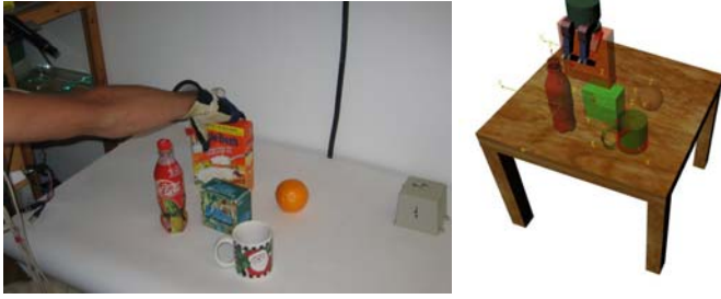
Fig. 9. Left: The human moves the rice box. The system recognizes what object has been moved and which grasp is used. Right: The robot grasps the same object using the mapped version of the recognized grasp.
